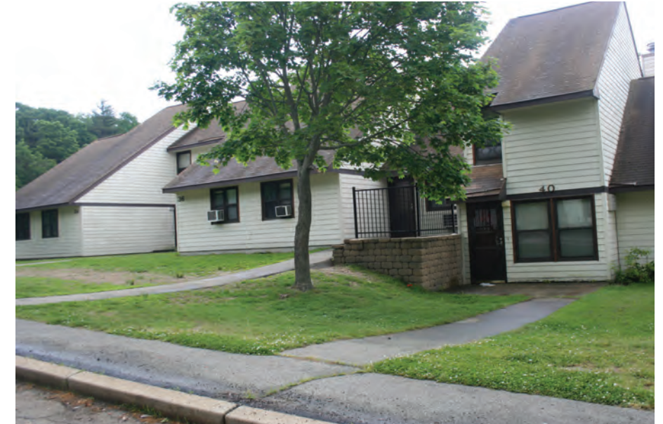
9. Most townhouses are at grade with a roll in entrance. The sloping landscape is accommodated with occasional retaining walls where buildings step down along with the topography.
